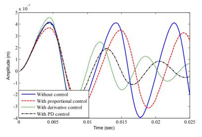
Figure 7 Vibration control of FG cylindrical shell using proportional, derivative and PD controller under mechanical loading (see online version for colours)
