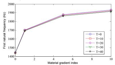
Figure 5 Variation of first natural frequency at various temperature gradients (see online version for colours)
