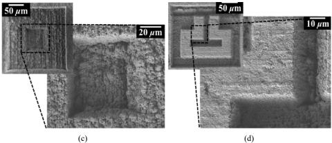
To confirm that the laser-fabricated microstructures were maintained after the thermal sintering process, we sintered zirconia green bodies micropatterned before and after debinding for 2 h at 1,400°C. The sintering process induced shrinkage of the pattern
