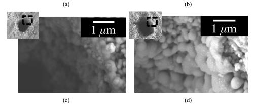
Figure 10 SEM images showing the behaviours of zirconia greenbody after debinding, corresponding to laser fluences of (a) 0.8 J/cm<sup>2</sup> (b) 1.9 J/cm<sup>2</sup> (c) 2.3 J/cm<sup>2</sup> (d) 3.9 J/cm<sup>2</sup>
