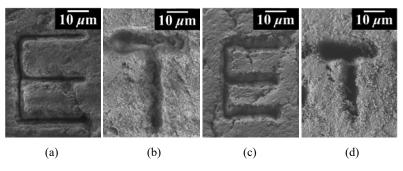
Figure 8 SEM images showing the cross-section of (a) bare bulk zirconia and bare zirconia greenbody (b) before and (c) after debinding
