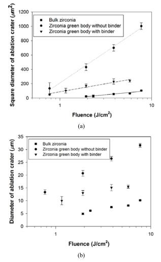
**Figure 3** (a) The dependence of  $D^2$  on lnF for evaluation of ablation threshold  $F^{\text{th}}$ , when N = 1,000 (b) Ablation diameter as function of fluence
