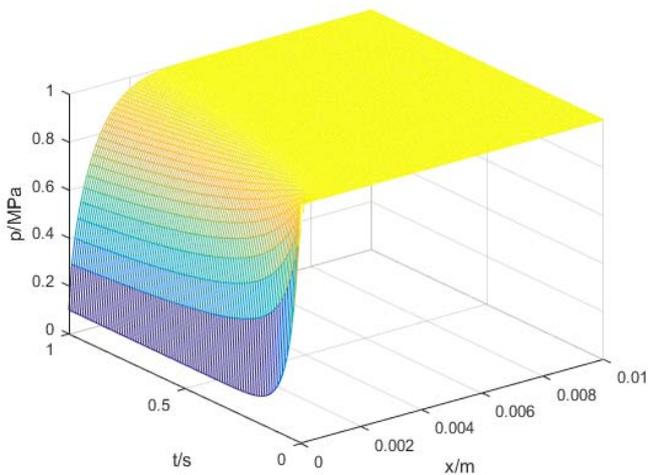
As shown in Figure 3, the maximum of correction pressure gradient appears at the position located in some distance from coal wall and a time delay. The time-space distribution characteristics of correction pressure gradient indicate that coal and gas outburst has the feature of losing its balance hierarchically.
