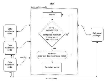
Data warehouse nodes scale-in is performed iff the average query execution time and the average load time respects the conditions (1) and (2) (where n represents the number of nodes):
