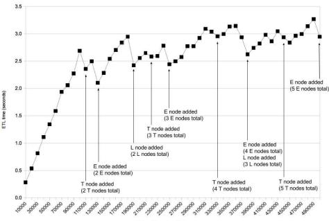
Figure 14 Near-real-time, full ETL system scale-out
