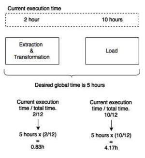
Another option is to configure both types of time bound limits: a global time bound for the entire ETL process and at the same time local bounds for the parts. In this case, AScale can use the local bounds to decide where to scale.
