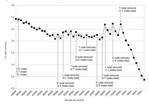
Figure 15 Near-real-time, full ETL system scale-in
