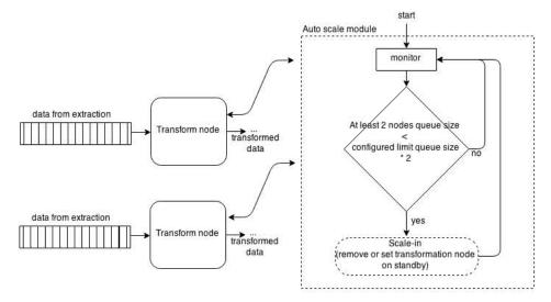
Figure 7 describes the algorithm used to scale-in. If queues size at a specific moment is less than half of the limit size for at least two nodes, then one of those nodes is set on standby (as ready node) or removed.
