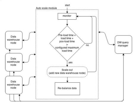
Data warehouse scalability is not only based on the load and integration speed requirements, but also on the maximum execution queries time. After a query is executed, if the query time is more than the configured maximum, then the data warehouse is set to scale-out. Figure 11 describes the algorithm used to scale-out the data warehouse based on the query execution time.
