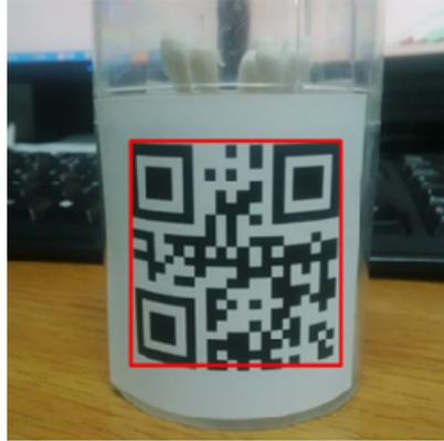
**Figure 8** Recognition test of CDPC on cylinder type object (see online version for colours)
