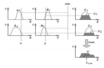
Figure 1 The Mamdani fuzzy interference system with min and max operators
