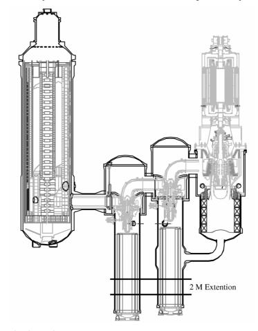
Figure 2 Extension of pre-cooler and inter-cooler to increase discharge water temperature
