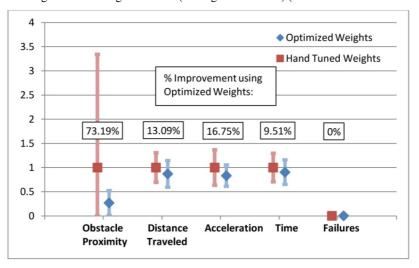
Figure 12 Comparison of normalised evaluation metrics between hand tuned and optimised weights for 10 design scenarios (one sigma error bars) (see online version for colours)
