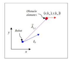
Figure 5 Configuration space representation of the robot and an obstacle (see online version for colours)
