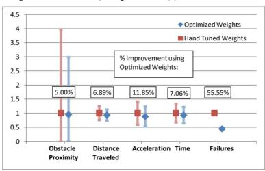
Figure 13 Comparison of normalised evaluation metrics between hand tuned and optimised weights for 1000 scenarios (one sigma error bars) (see online version for colours)
