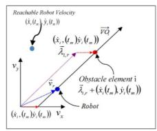
In this paper, it is assumed that the relative position and velocity of the goal are known. As such, locating and tracking the centre of certainty is not needed to find the *velocity* goal,  $\overline{VG_i}$ , or the set of robot velocities which will lead the robot to the goal, in the same manner that the velocity obstacle was found. However, if a sensor was employed that could distinguish the goal from surrounding obstacles, then the same technique used for
