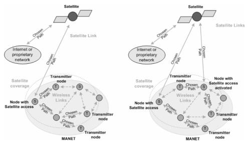
**Figure 7** Hybrid MANET-satellite network challenge: resource management – automatic access point activation to increase throughput
