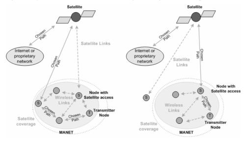
Figure 5 Hybrid MANET-satellite network challenge: selecting satellite access points
