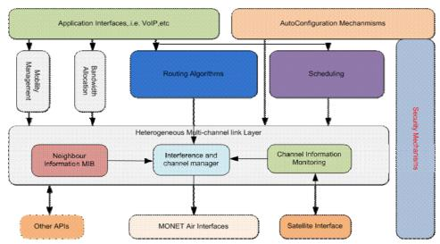
The MONET has developed the architecture to optimise the integration of satellite links in a MANET network. The complementary roles of the satellite segment and the wireless ad hoc network should enable the provision of high communication capability, broadband communication, reach back and interconnection of several ad hoc networks. The following are the main functions of the architecture:
