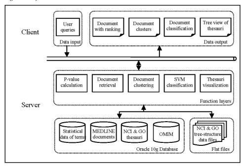
Figure 5 System architecture
