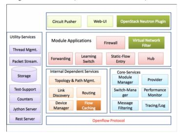
Figure 2 Floodlight controller structure (see online version for colours)
