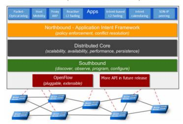
Figure 1 ONOS controller structure (see online version for colours)
