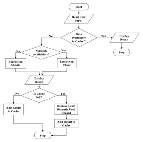
The resource intensive job of the application is executed on cloud server on network availability else execution happens on mobile device. If any one of the cloud servers fails, the execution will be migrated to the next optimal cloud. MCDA techniques are used to find the optimal cloud from a class of four cloud servers positioned in different regions. The criteria and alternatives required for cloud path selection can be changed as per the developer requirement.
