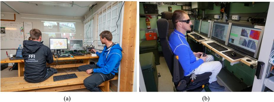
In the operation centre in the stationary container two operators used the OCUs from GVSC and PIAP. On the wall a projector displays a video feed from each robot. The video feed was set up using GStreamer, in order to have a low latency viewer for the streams. A screen showing the location of all the robots in a map was also set
