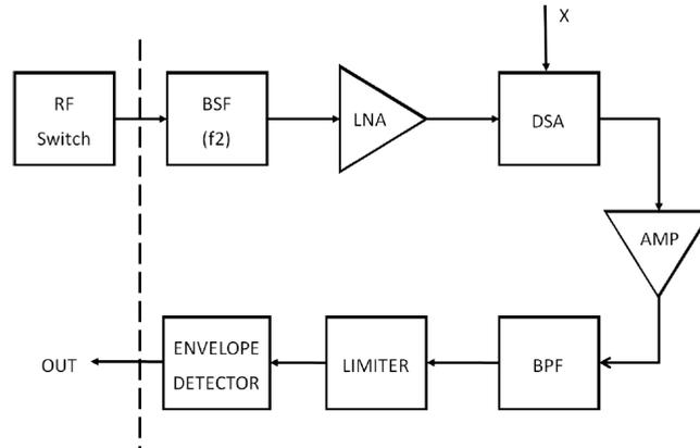
**Figure 9** Block diagram showing frequency propagation for transceiver 1
