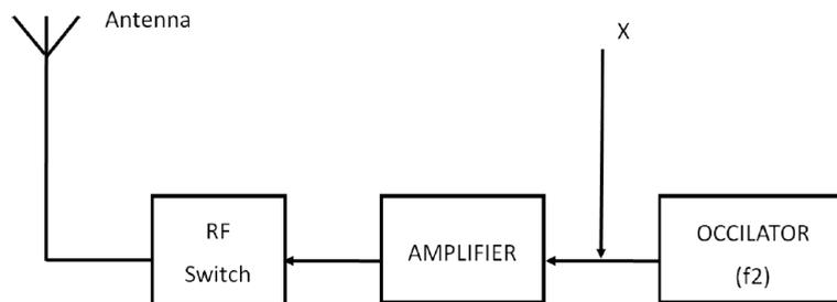
The amplitude shift keying (ASK) modulated pulse requires an ON time of 2 micro sec, with a frequency of 10 kHz. ASK signal produced should have a power level of 10 dBm when ON, and during OFF, the power level should be  $< -90$  dBm. The pulsed RF signal from transmitter is shown in Figure 7.
