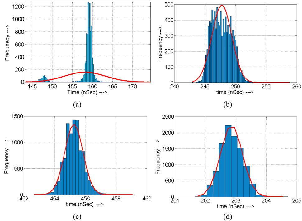
The results using only active radar and enhanced active radar have been compared. Figures 20(a) and 20(b) show the measurement result with active radar without using the BSFs. It can be seen that the standard deviation for the measurement is quite large as compared to the Figures 20(c) and 20(d), where enhanced active radar with frequency shift was used, thus enabling to measure distance much precisely.
