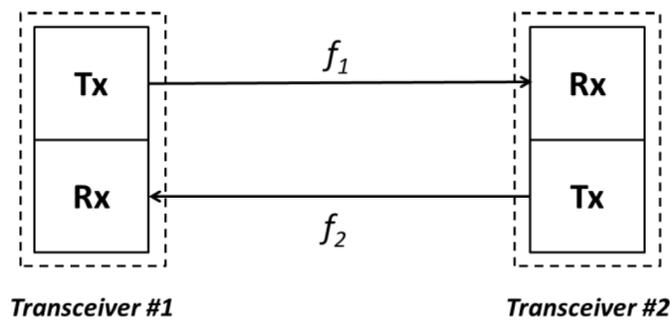
In the active mode of radar operation, the master accepts only the active encoded data sent by the slave, neglecting all echoes generated by any number of obstacles present in the path. This clearly mitigates the obstacle problem mentioned previously. The above
