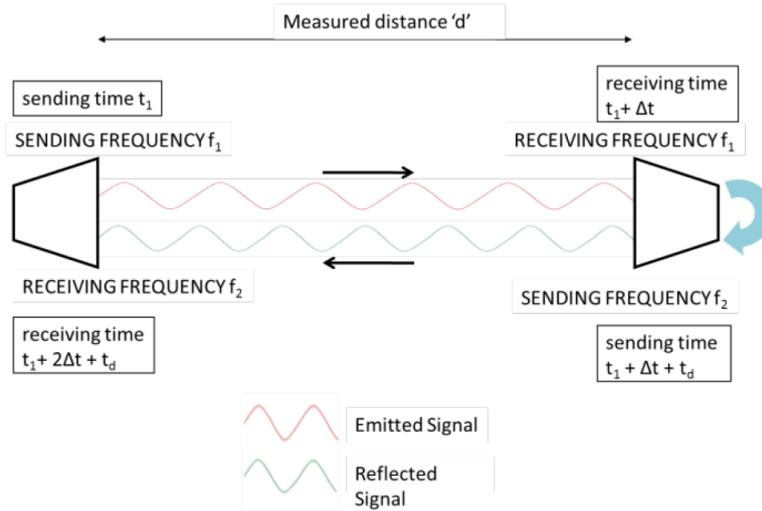
**Figure 5** The frequency link between transceiver #1 and #2
