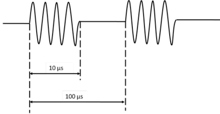
The maximum range at which a target can be located that the leading edge of the received backscatter from that target is received before transmission begins for the next pulse. This range is called maximum unambiguous range or the first range ambiguity. The pulse-repetition frequency (PRF) determines this maximum unambiguous range of given radar before ambiguities start to occur. This range can be determined by using the following equation:
