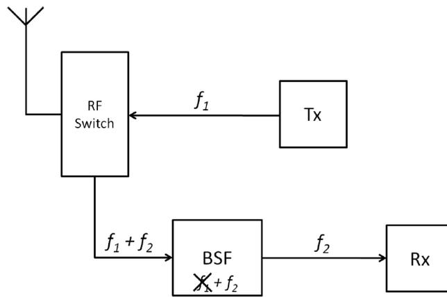
**Figure 10** Block diagram showing frequency propagation for transceiver 2
