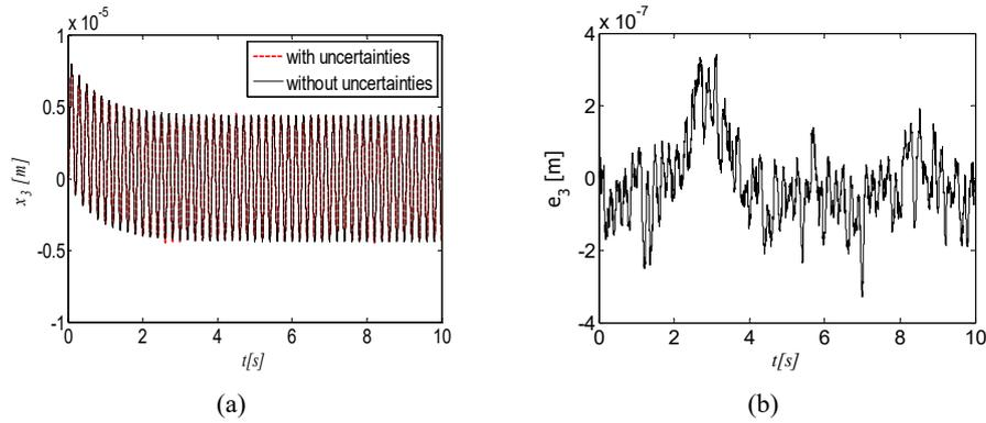
In Figure 9 we observe the robustness of the control where  $|e_a| = |\dot{x}_4 - \hat{\dot{x}}_4|$  represents the acceleration deviation obtained by control without uncertainties ( $\dot{x}_4$ ) and acceleration obtained by control with parametric uncertainties ( $\hat{\dot{x}}_4$ ), and  $|e_u| = |u - \hat{u}|$  represents the signal control obtained by control without uncertainties ( $u$ ) and signal control with parametric uncertainties ( $\hat{u}$ ).
