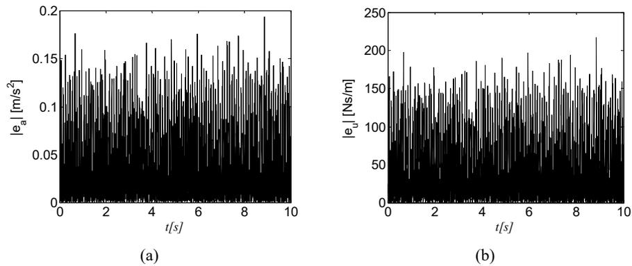
As can be seen in Figure 9, the proposed control is not sensitive to errors in the parameters of the matrix  $A$ , maintaining the level of acceleration and displacement below the uncontrolled system. As the acceleration in rms for the parametric error case is  $(\ddot{x}_{3_{rms}} = 0.0449[m/s^2])$ , it is possible to note that occurred a reduction of approximately (83.456%) relative to system without control, and the error was  $e_{3_{rms}} = 1.0729 \times 10^{-7}[m]$  in rms.
