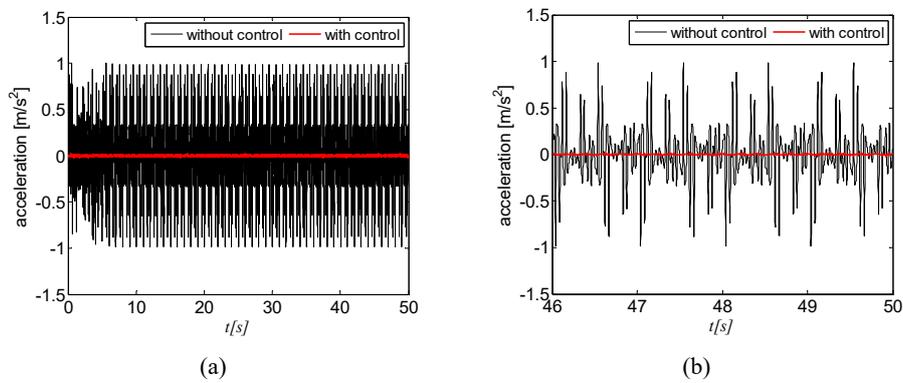
It is possible to observe that the proposed control reduces the system oscillation amplitude (Figure 5). The rms of the magnitude acceleration peak has been reduced in about 98.6367% (Figure 6), where the uncontrolled system acceleration ( $\ddot{x}_{3ms} = 0.2714$ ) was reduced to ( $\ddot{x}_{3ms} = 0.0037$ ) when the MR damper was introduced into the system.
