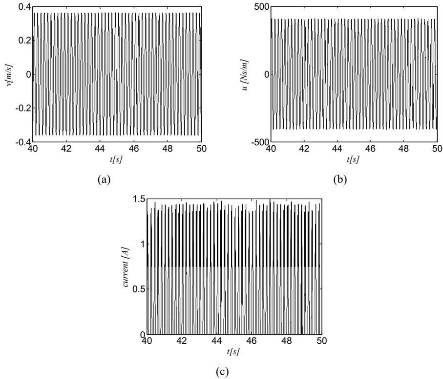
As shown in Figure 7(b), the value of the force control is less than 420 Ns/m, being a common value of the force developed by MR dampers. Also we can see in Figure 6(c), the electric current required to control the MR damping force.
