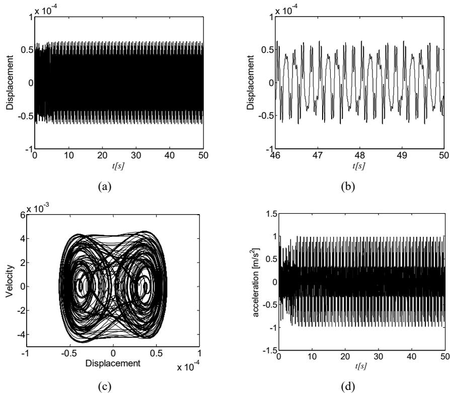
Here, scale index was obtained using the Daubechies eight-wavelet (db8) function and the scale interval from  $s_0 = 1$  to  $s_1 = 512$ . As can be seen from the figure that the displacement of ( $x_3$ ), has a non-periodic behaviour comproved by the index scale ( $i_{scale} = 0.1134$ ), and the acceleration which passengers are exposed is close to  $1.02[m/s^2]$ .
