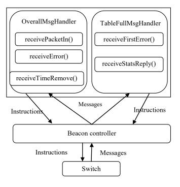
A TableFullMsgHandler is implemented to evict useless and malicious rules from the flow table in order to mitigate the overflow of the flow table.
