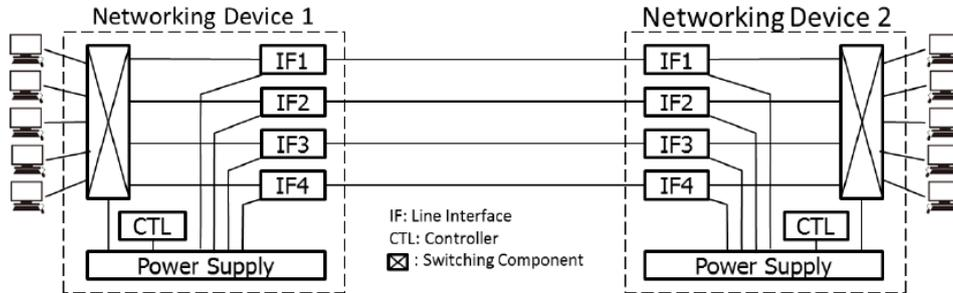
Figure 9 Power saving scheme by lulling line interfaces to sleep
