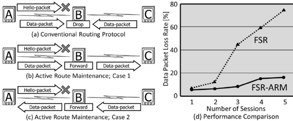
In order to investigate the effect of this technology, comparative experiments of the proactive type routing protocol, i.e., fisheye state routing (FSR) (Gerla and Hong, 2002) and FSR-ARM which implemented the proposed ARM mechanism in FSR, were
