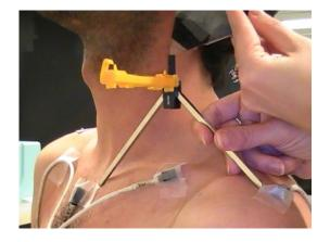
Figure 3 This custom-designed triangular reference frame with bubble level was used to find the third point of the clavicle (see online version for colours)
