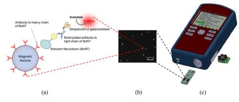
Notes: The bright wells correspond to a single enzyme label associated with a bead. All bead incubations, washing, array loading, and imaging occurs on a microfluidic chip. A handheld reader images the arrays, and a reagent cartridge houses beads and labelling reagents.
