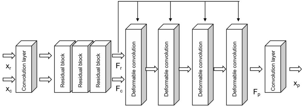
Firstly, the feature extraction module is used to map the input reference frame and the current frame ( $X_C$ ,  $X_R$ ) to its feature domain ( $F_C$ ,  $F_R$ ) to make full use of high-order motion features to learn more accurate motion offset. The feature extraction module is usually composed of a  $3 \times 3$  convolution layers and three residual learning blocks.  $K$  pixels through convolution operation, expressed as:
