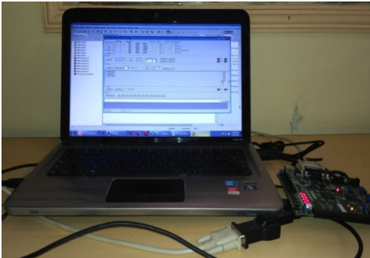
Figure 4 Real time execution of adaptive noise canceller on Nexys 2-500 SPARTAN 3 Development Board (see online version for colours)
