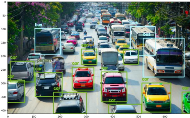
Figure 12 Vehicle detected by the program feed in the system (see online version for colours)
