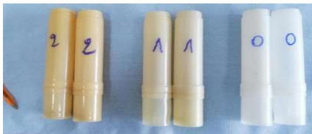
Figure 1 The polyethylene shuttles numbered 0 not irradiated, 1 irradiated once and 2 irradiated twice (see online version for colours)
