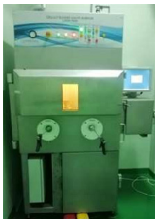
Figure 2 Shielded cell for the handling and cooling of shuttles (see online version for colours)
