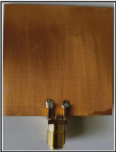
Figure 4 Fabricated prototype antenna bottom (see online version for colours)
