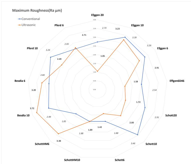
**Figure 18** Comparison of minimum and maximum roughness for conventional and ultrasonic assisted machining (see online version for colours)
