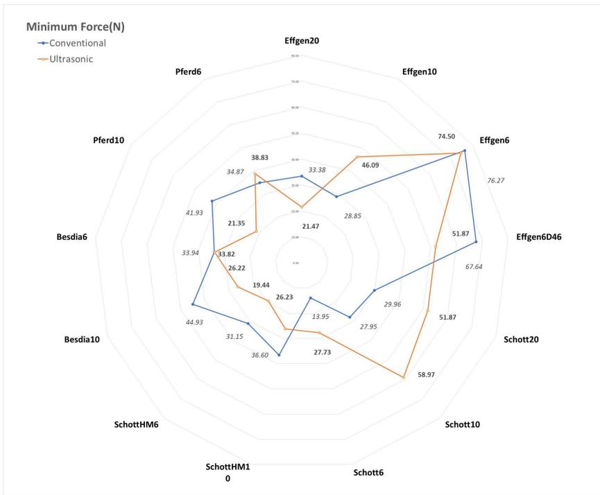
**Figure 12** Comparison of maximum forces for conventional and ultrasonic assisted machining (see online version for colours)
