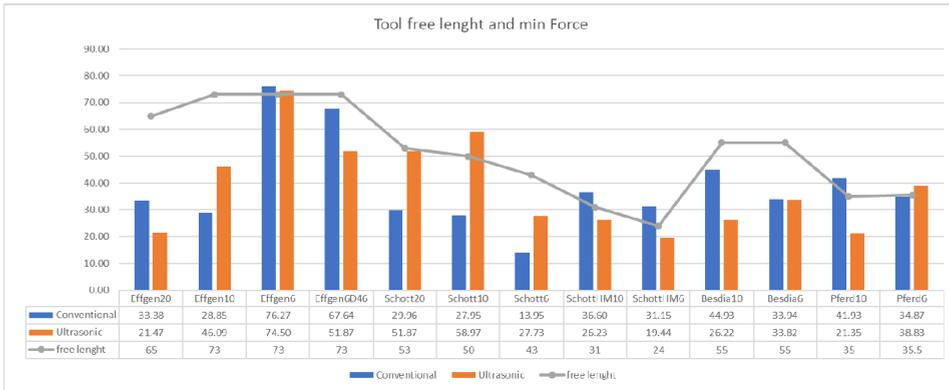
In addition, after comparing the ratio of the tool free length per diameter of the tool and reverse ratio the previous conclusion was achieved and 62% of the results coincided with the theoretical results (Figure 15).
