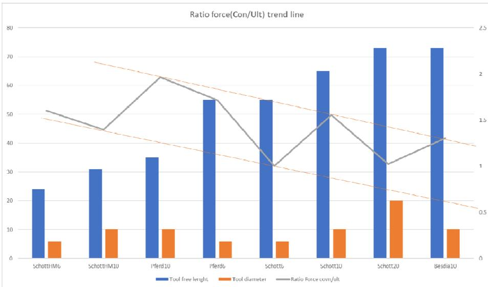
It can be considered that the results for eight of the thirteen tools (62%) have coincidence with theory. After sorting the tools according to the length, the trend lines show that with increasing the free length, tool ratio force (conventional per ultrasonic) is descending. That means the vibration and other variables are influencing the stability of the tools. It
