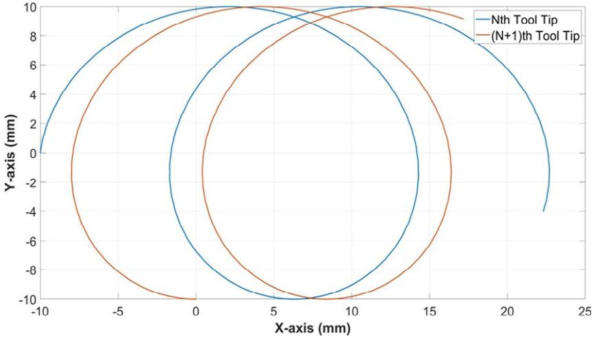
**Figure 2** Cutting tool tip movement of axial (Z-direction) vibrated UVAM (see online version for colours)
