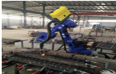
Figure 3 Actual working condition of sample welding robot (see online version for colours)
