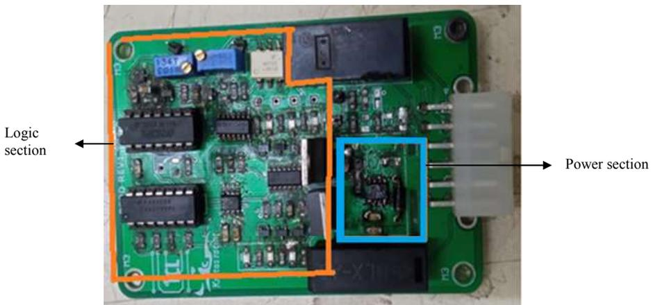
Figure 26 shows the assembled board of ECU 1 PCB on which there is an STM32 microcontroller, APPS control circuit, and RTDS.
