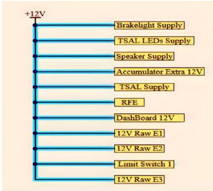
Figure 19 shows the fused supply to different circuits via PDU.
