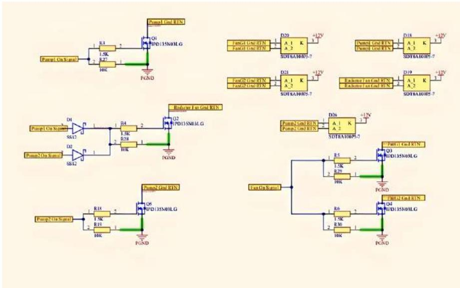
Figure 20 illustrates the cooling supply and control system, while Figure 21 displays the current and voltage sensing components. The ASC712 current sensing IC is employed to detect battery current, and a voltage divider is utilized to measure battery voltages.
