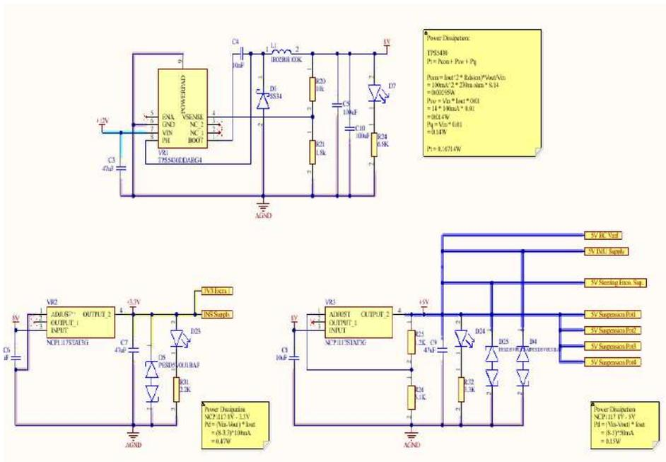
Figure 18 shows the unfused supply to different circuits via PDU.
