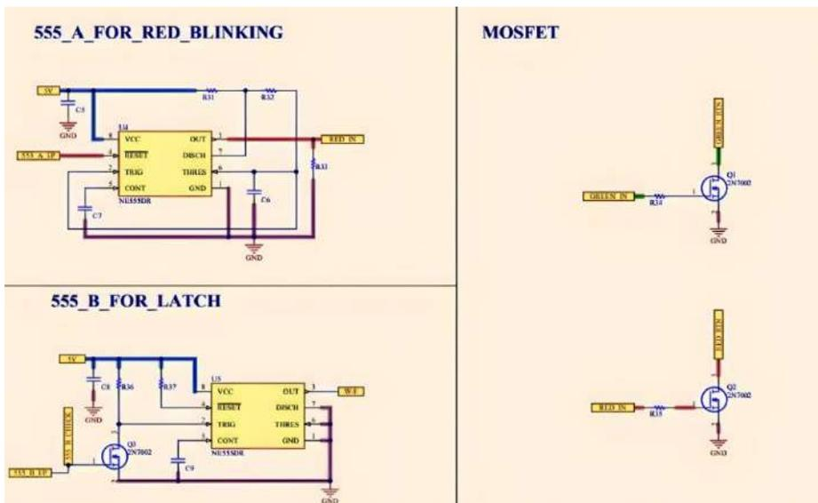
The wire fault detection circuits depicted in Figure 8 are engineered to detect and address wire faults in the accumulator isolation relay and precharge state signal wires.
