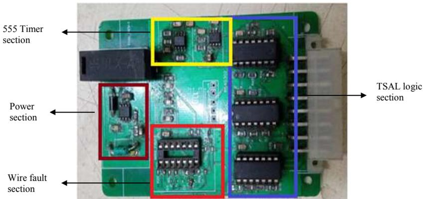
Figure 25 shows the assembled board of BSPD PCB on which there are 2 logic gates, 1 relay, TPS5430 voltage regulator, Op-amp, etc.
