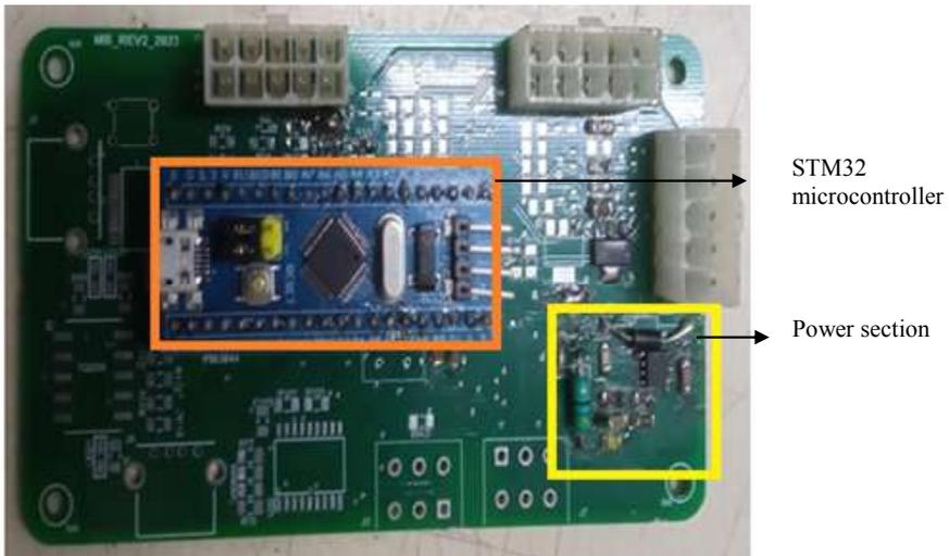
Figure 27 shows the assembled board of ECU 2 PCB on which the latching circuit is relays.
