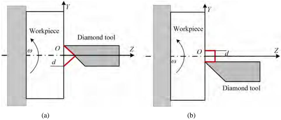
**Figure 3** Eccentricity error in X-direction for turning convex surface, (a) inner eccentricity and (b) outer eccentricity of the convex surface
