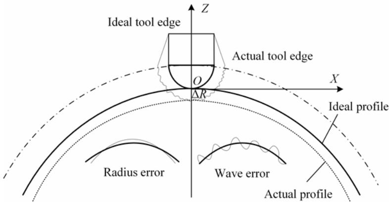
3.4 Profile error compensation based on B-axis
