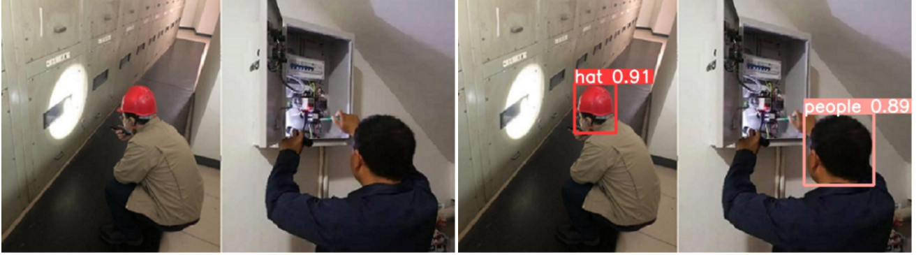
Figure 6 Detection examples of the safety helmet wearing detection model for distribution room operators (see online version for colours)
