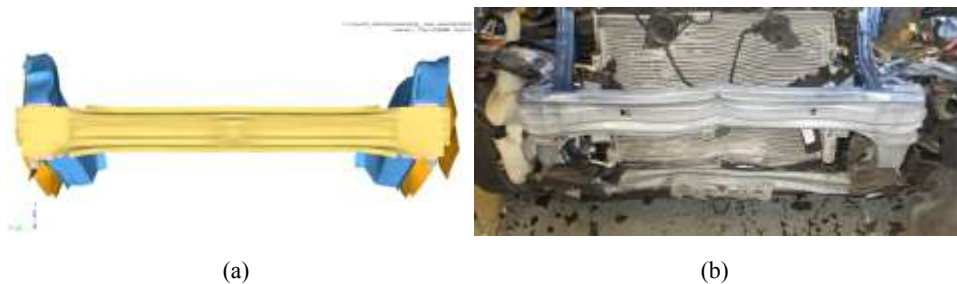
Figure 3 Deformation of simulation and test: (a) simulation and (b) test (see online version for colours)
