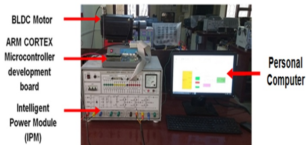
Figure 18 Experimental set up and its related instrumentation (see online version for colours)
