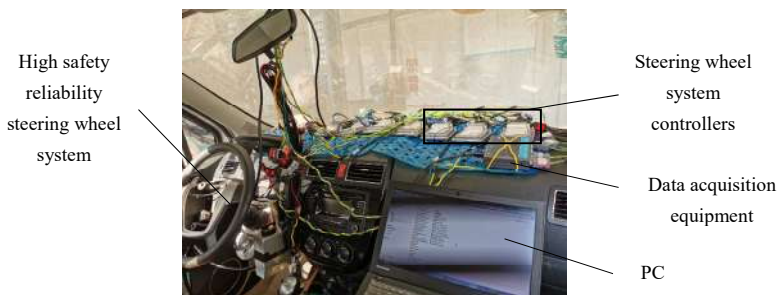
Figure 14 Steering wheel system with high safety reliability vehicle test platform (see online version for colours)
