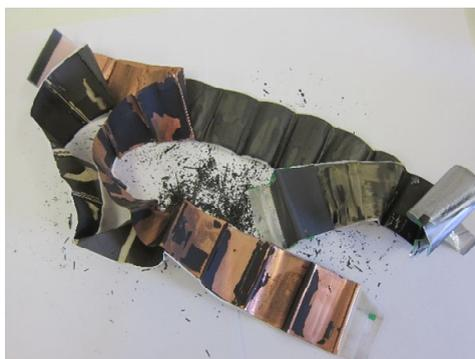
This study was firstly undertaken by manual dismantling of the batteries to perfectly know the composition of the active cathode materials used nowadays in the market and, with such information, be able to design the best physical separation process to reach the goal of this research.
