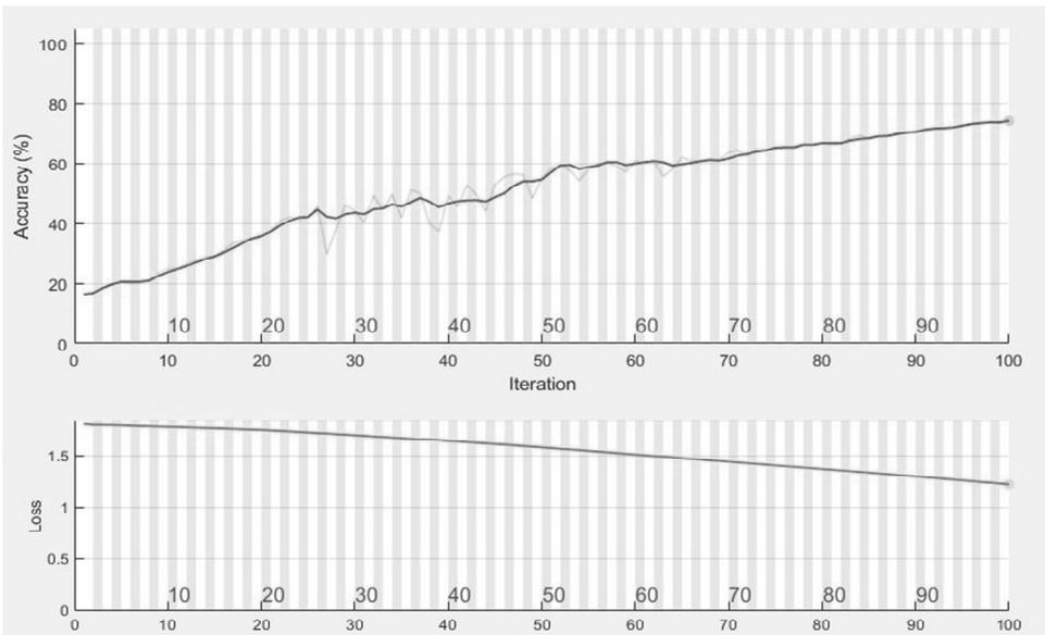
As training progressed, training loss decreased and training accuracy increased. When training finished, the ANN training accuracy was higher than 74%. Network testing accuracy was 69.4% when tested using the testing set.
