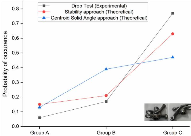
From the CSA method values are plotted in the graph and the result is shown in Figure 10. In this method also, the most probable orientation is identified as the group C-like stability method. The drop test in different heights from 100 mm to 950 mm in the interval of 50 mm and the probability of occurrence of each group is presented in Figure 10. From the drop test results, group C orientation is identified as the most probable orientation when compared to other orientations.
