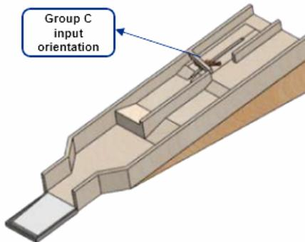
If the rocker arm drops initially in group C orientation (shown in Figure 15), it will move leftward because a protrusion on top of the component will be struck by the wiper blade. The continuous vibration moves and slides the part leftward until reaching its end at the feeder which remains in group C orientation. Table 3 shows the time taken for the part to change its input orientation to group C orientation.
