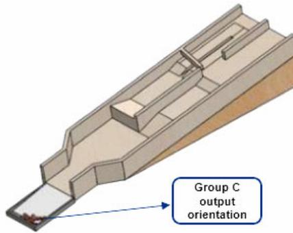
In the motion analysis process, initially, when the rocker arm is dropped in group A, B, or D orientation (as shown in Figure 16), the rocker arm travels through the slotted path and goes under the wiper blade, after which the rocker arm travels upon riser to change its final orientation to group C which is shown in Figure 17.
