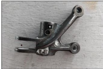
**Figure 3** Possible orientations of the modified rocker arm
