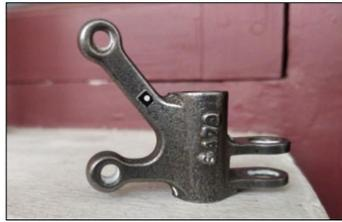
**Figure 2** Rear view of the modified rocker arm
