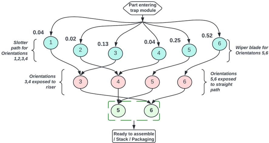
The slotted route is accessible to all dropping orientations after the initial stage of the portion at the trap module. Orientations 1, 2, 3, and 4 travel via the slotted route, whereas orientations 5 and 6 are exposed to the wiper blade due to the component’s projected surface. So 5 and 6 orientations travel a different path, while 1, 2, 3, and 4 orientations are exposed to the riser to further shift the orientation to group C orientations.
