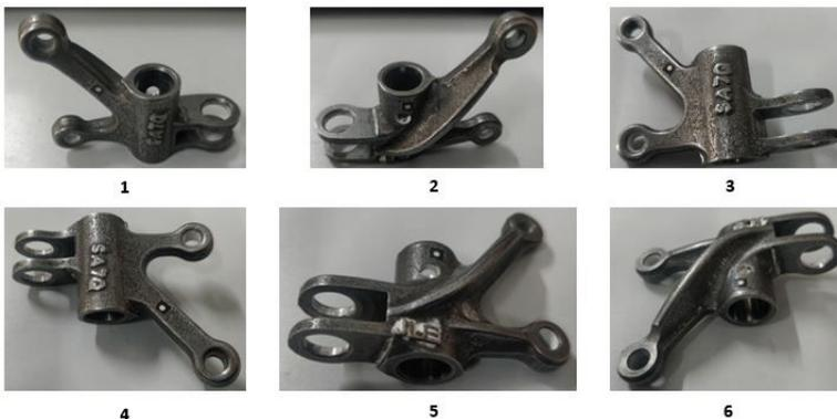
The possible orientations of the modified rocker arm are shown in Figure 3. The number of possible orientations for the selected rocker arm component is six and there exist some non-possible orientations also but they are not considered. Typically orientation of the part is based on the geometry of the part while for the rocker arm; the number of possible orientations is six.
