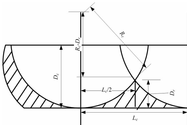
Fly cutting surface profile was generated through the tool sweeping movement across the workpiece surface, as shown in Figure 2,  $D_c$ ,  $L_c$  and  $R_c$  are cutting depth, feed step size and tool radius, respectively. According to the geometric relationship illustrated in Figure 2, the residual height  $D_r$  could be expressed as equation (1) without considering the kinematic motion errors.
