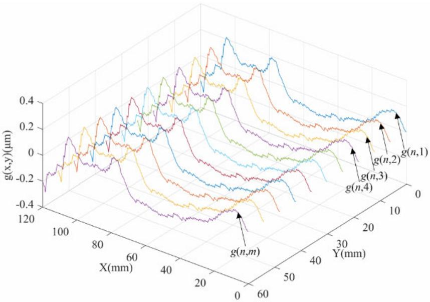
**Figure 7** Guideways straightness surface overlying map (see online version for colours)
