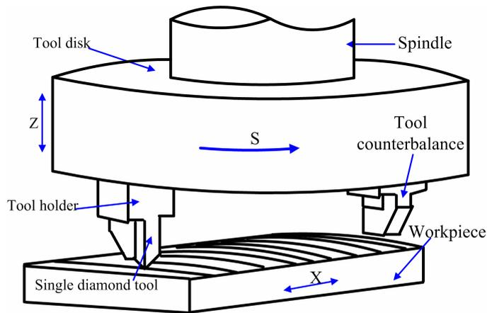
**Figure 2** Residual height generating model
