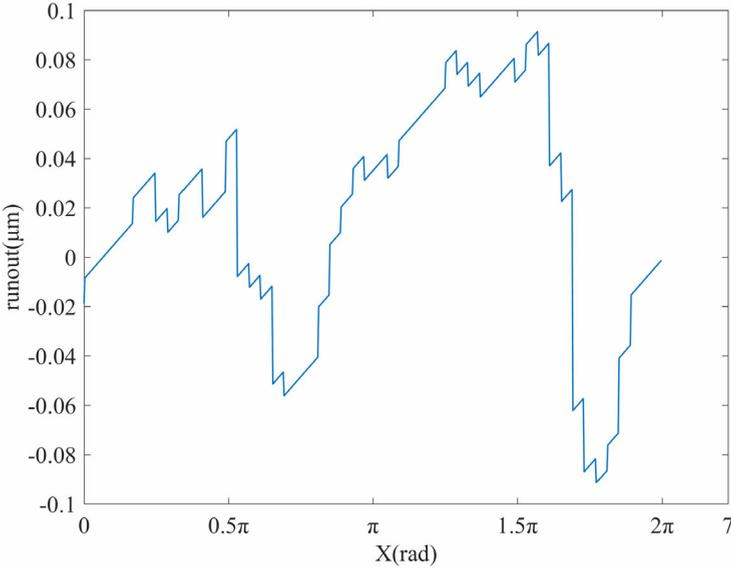
**Figure 9** Spindle axial runout line overlying map (see online version for colours)
