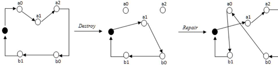
As Figure 3 shows, by applying destroy operators, customers  $a_0$  and  $a_2$  are removed which turns the solution to a partial solution. The repair operator aims to reconstruct this partial solution to make it complete by inserting the destroyed customers:  $a_0$  and  $a_2$ . In our ILSFC-SP approach, we used random removal as a destroy operator and the greedy insertion to repair the solution.
