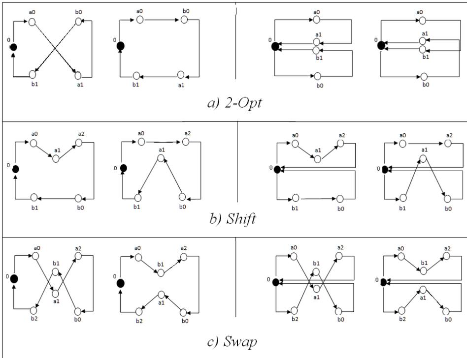
The different moves in inter-route (right side) and intra-route (left side) modes are introduced in Figures 2(a), 2(b) and 2(c) where node 0 indicates the depot. In
