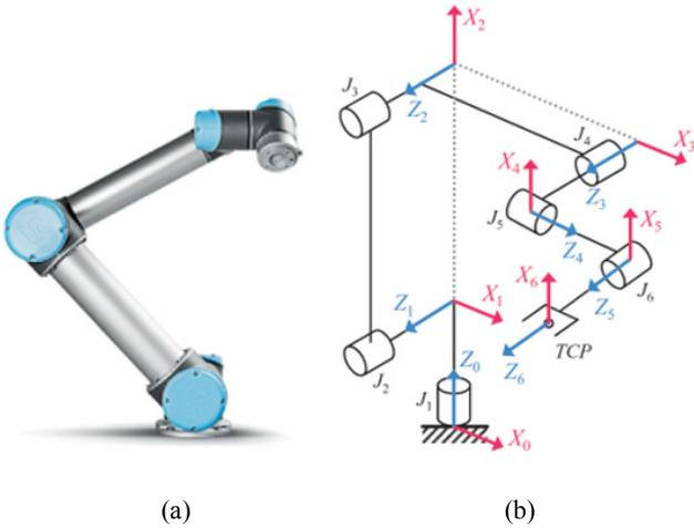
$a_i$ : the distance along  $X_i$  from the intersection of the  $X_i$  and  $Z_i$  axes to  $O_i$  (if  $Z_i$  intersects  $Z_{i-1}$ , locate  $O_i$  at this intersection; if  $Z_i$  and  $Z_{i-1}$  are parallel, locate  $O_i$  in any convenient position along  $Z_i$ ).
