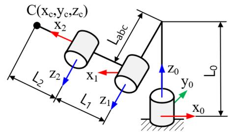
**Figure 4** Inverse kinematics calculation procedure
