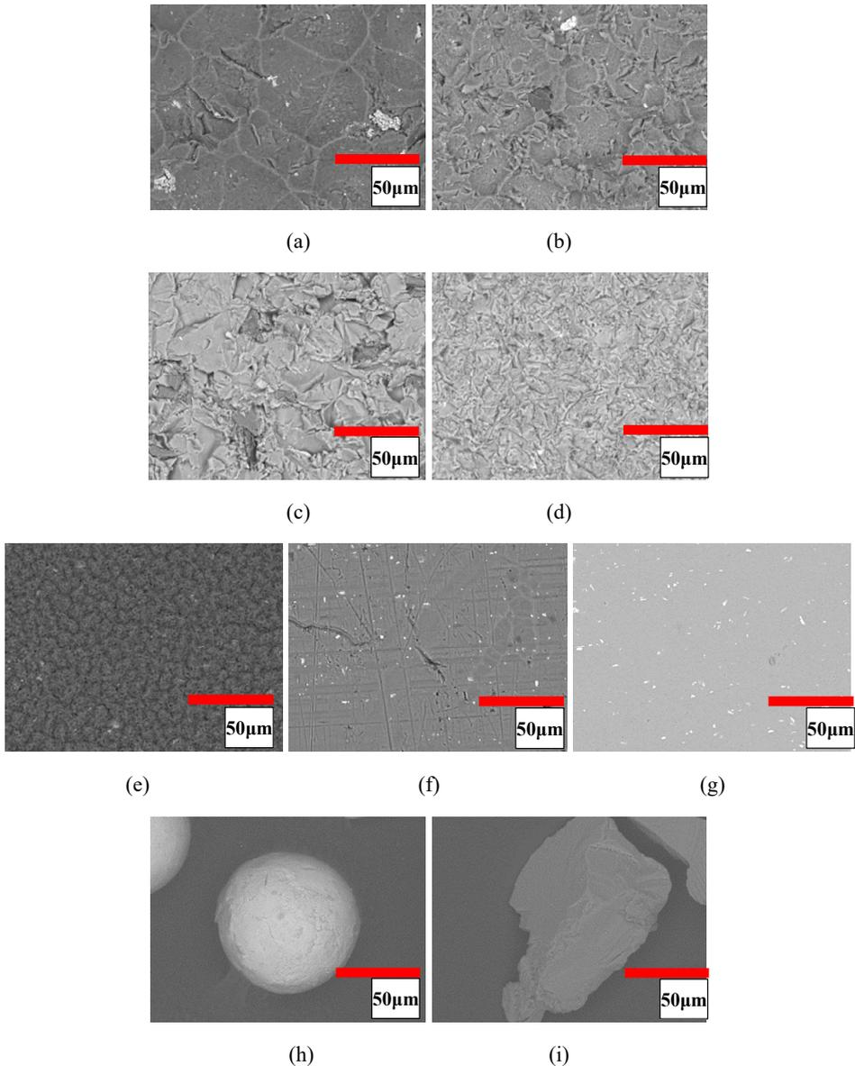
**Figure 2** Shape of projectiles (average diameter), (a) steel particles (60  $\mu\text{m}$ ) (b) steel particles (25  $\mu\text{m}$ ) (c) WA particles (80  $\mu\text{m}$ ) (d) WA particles (20  $\mu\text{m}$ ) (see online version for colours)
