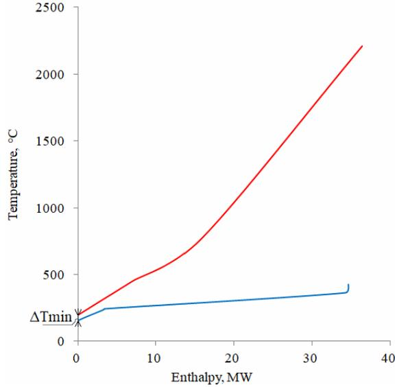
**Figure 5** Converted heat flows of the furnace in the ‘exergy-temperature’ coordinate system (see online version for colours)
