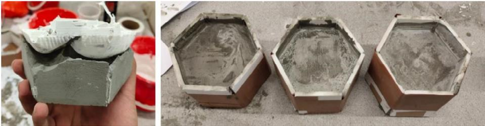
Notes: Illustration of home-produced prototypes using 3D Printed formwork and Concrete. Students develop their designs digitally and use rapid prototyping fabrication services that can deliver materials direct to their home. This material is then used for the manual creation of original works as cast prototypes.
