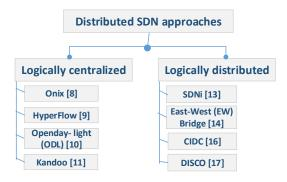
Although HyperFlow and Onix allow the distribution of the SDN control plane, they produce a lack of flexibility and scalability limitation.
