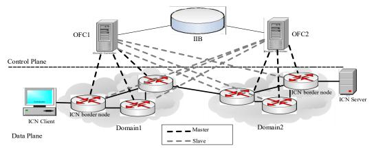
The synchronisation between different controllers is performed thanks to the shared IIB. The controller decisions are taken by the control plane on the basis of data plane events while the consistent network state is performed through the IIB due to the communicated information such as read and write operations.
