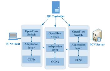
To achieve our goal, we exploited the master-slave configuration defined in OpenFlow 1.3 (Pfaff et al., 2012), which allows switches to tolerate controller crashes thanks to its ability of connection to more than one controller. In our design, the primary controller of one domain presents the backup controller of another domain to provide controller fault tolerance as depicted in Figure 4.
